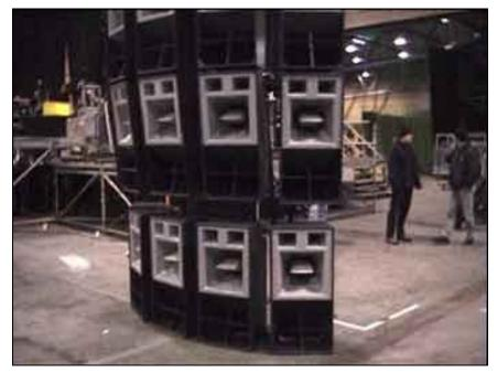
The array can then raised again ready for the next row of Resolution enclosures
