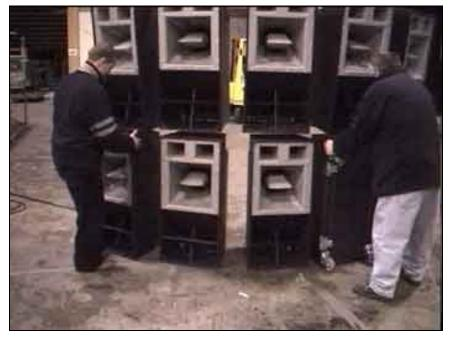
Next, raise the grid and arrange the next row of cabinets underneath
