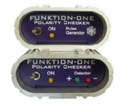
The ASPC1 is a two-part system comprising a pulse generator and a detector. The pulse generator allows you to inject a special test signal anywhere in the signal path whilst the detector microphone lets you check the resulting loudspeaker polarity acoustically. See the ASPC1 user guide for more information.
