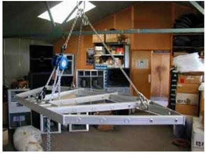
Each spoke of the grid is fixed at the optimal horizontal splay angle of 20 degrees
