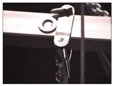
Attach tilting straps to the grid using the smaller version of the sword pin (on a special fitting that forms part of the strap)
